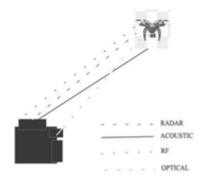
Figure 1. Existing Micro-Drone/UAV detection system
